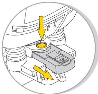
Press the red button and pull the slide lock back away from seat.
