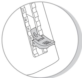
Lift lever to adjust height of footrests.
