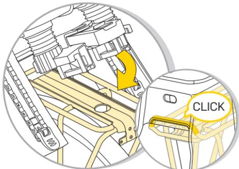
Hook seat onto front rail of rack. Rotate seat down on rack surface until snapped into positive engagement.
