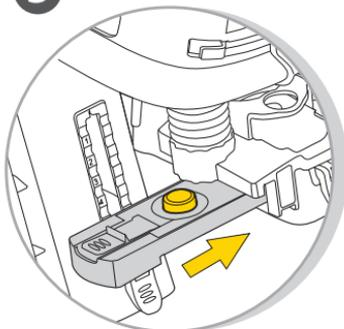
Press red button and push slide lock back into rack.
