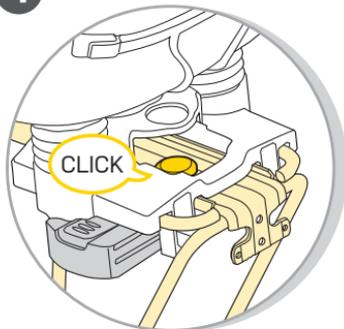
Make sure positive engagement "click" is heard and red button is protruding through hole in rack surface.
